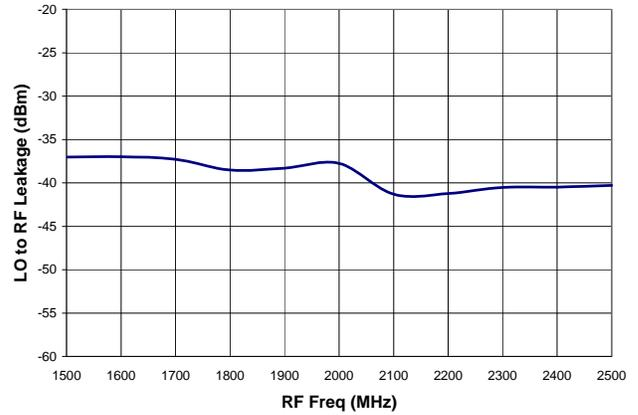
Figure 7. LO to RF Leakage versus LO Frequency
